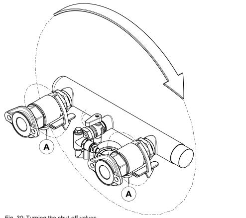
Fig. 30: Turning the shut-off valves
