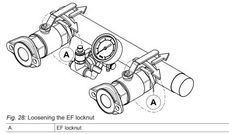
7. Undo the EF locknut at both shut-off valves by half a turn. The O-ring is now exposed.
