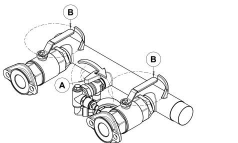
Fig. 29: Turning the pressure measuring set
