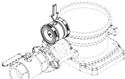
Fig. 22: Mounting the body
