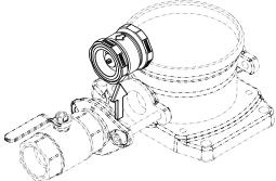
Fig. 21: Removing the body
