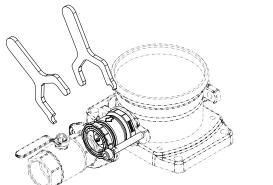
Fig. 20: Screwing the valve's body parts into each other
