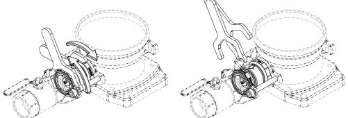
Fig. 23: Loosening the screwed connection of the body parts
