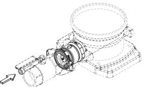
Fig. 25: Fitting the screw
