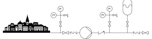
*Fig. 3:* M = Inlet side of pressure booster system connected to the municipal water supply, suction head operation
