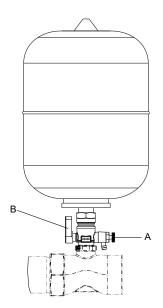
Fig. 13: Venting and draining the accumulator
