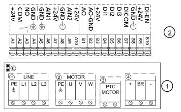
Fig. 11: Overview of terminal strips for variant with 1 relay
