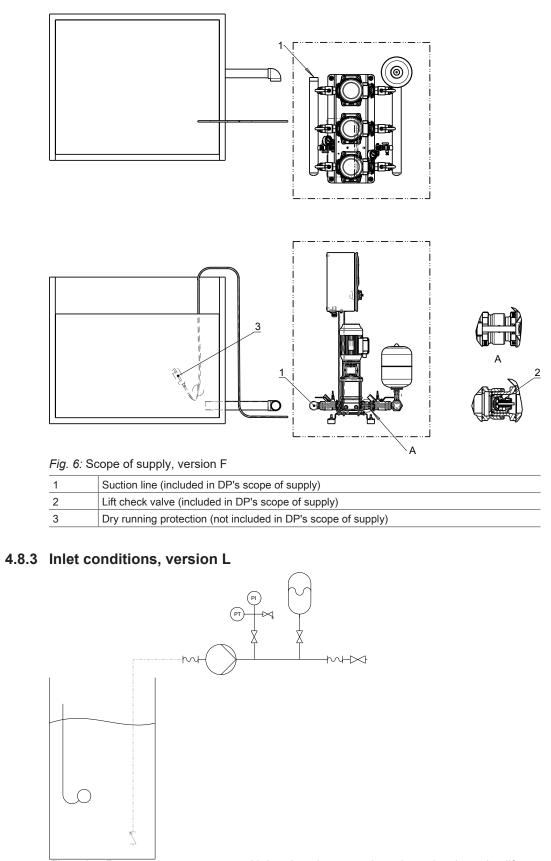
*Fig.* 7: L = Pressure booster system with break tank arranged at a lower level, suction lift operation
